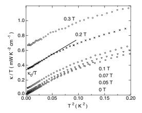
Fig. 1.  $\kappa/T$  vs  $T^2$  for NbSe<sub>2</sub>. The line shows the  $T \to 0$  extrapolation which yields the electronic contribution  $\kappa_0/T$ . In zero field,  $\kappa_0/T = 0$ , as expected for a superconductor without nodes in the gap anywhere on the Fermi surface.
