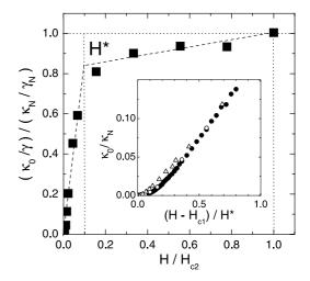
Fig. 3. Field dependence of  $\kappa_0/\gamma$  (main panel). The inset shows the field dependence of thermal conductivity for NbSe<sub>2</sub> (circles) and V<sub>3</sub>Si (triangles), plotted as a function of  $(H - H_{c1})/H^*$  where  $H^* = H_{c2}/9$  for NbSe<sub>2</sub> and  $H^* = H_{c2}$  for V<sub>3</sub>Si.
