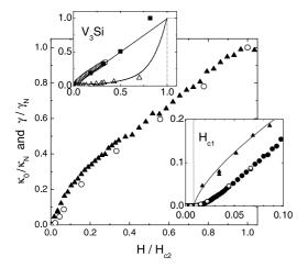
Fig. 2. Field dependence of thermal conductivity (circles for NbSe<sub>2</sub> and empty triangles for  $V_3Si$ ) and specific heat (filled triangles for NbSe<sub>2</sub> and squares for  $V_3Si$ ) in NbSe<sub>2</sub> (main panel and lower inset) and  $V_3Si$  (upper inset). The filled circles come from a field sweep at 100 mK. Both quantities are normalized to the values in the normal state.
