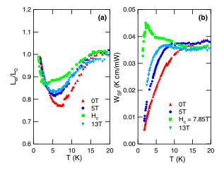
FIG. 4 (color online). (a) Temperature dependence of the electronic contribution to the Lorenz ratio L(T), which is consistent with the standard picture for itinerant electron metamagnetism. (b) The thermal resistance  $W_{\rm SF} \equiv 1/\kappa_{\rm el} - \rho_0/L_0T$  attributed to scattering off of spin fluctuations.
