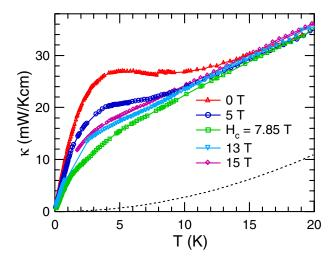
FIG. 1 (color online). High temperature thermal conductivity at several fields along the c axis including the critical field. The heat current was applied in the ab plane. The dashed line is an estimate of the phonon conductivity obtained by considering the WFL as discussed later in the text.
