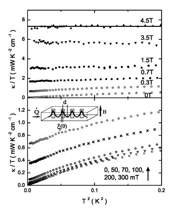
FIG. 1. Thermal conductivity of NbSe<sub>2</sub> at several applied fields, plotted as  $\kappa/T$  vs  $T^2$ . The solid line indicates the value expected from the Wiedemann-Franz law as obtained from resistivity measurements at H=4.5 T. The field is applied parallel to the c axis and perpendicular to the heat current  $\dot{Q}$ .
