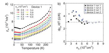
FIG. 2 (color). (a) Longitudinal resistivity  $\rho_{xx}$  of device 1 as a function of temperature at different carrier densities tuned by the back gate. (b) Slope of  $\rho_{xx}$  vs carrier density in the linear temperature regime (50 K < T < 150 K). The dashed line indicates the high carrier-density value of the slope used to compare to the theoretical model.
