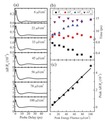
FIG. 4. (Color online) Panel (a) shows the peak differential reflection signal (x = y = 0) as a function of the probe delay with different pump fluences, as indicated in each plot. Panels (b) and (c) summarize the characteristic times and the peak of the signal as functions of the pump fluence.
