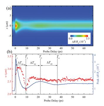
FIG. 2. (Color online) Panel (a) shows the differential reflection signal as a function of the probe delay and x, measured with y=0. Panel (b) shows the peak differential reflection signal (x=y=0) as a function of the probe delay (solid line, right axis). The squares (left axis) show the width (FHWM) of the profile as a function of probe delay, obtained through a procedure shown in Fig. 3.
