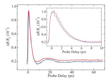
FIG. 6. (Color online) The peak differential reflection signal (x = y = 0) as a function of the probe delay with different pump spot sizes of 3  $\mu$ m (blue/lower) and 11  $\mu$ m (red/upper), respectively. The energy fluence of the pump pulse at the center of the spots is 17  $\mu$ J/cm² for both measurements. The inset shows the two curves at early probe delays.
